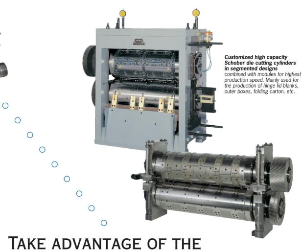
TAKE ADVANTAGE OF THE ADVANCED SCHOBER ROTARY DIE CUTTING, CREASING AND PUNCHING TECHNOLOGY
