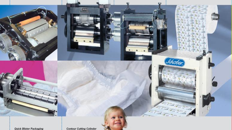
Built in module in round design with rotary punching tools for line hole or registration hole punching into multilayer, difficult to process material.
